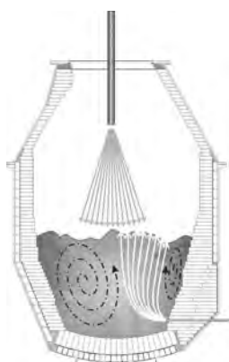
Fig. 2. Schematic presentation of an AOD converter. It should be noted that the ferrochrome converter is geometrically very similar to AOD presented in this figure.
